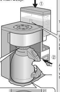
Align the slot on the Water Tank with the tab on the Main Body
