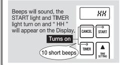
The Automatic Shut-Off function activates to shut off power to the heater in order to prevent damage from overheating. The Display will show "HH" to alert you that the Automatic Shut-Off has been activated. The following conditions may cause activation:
